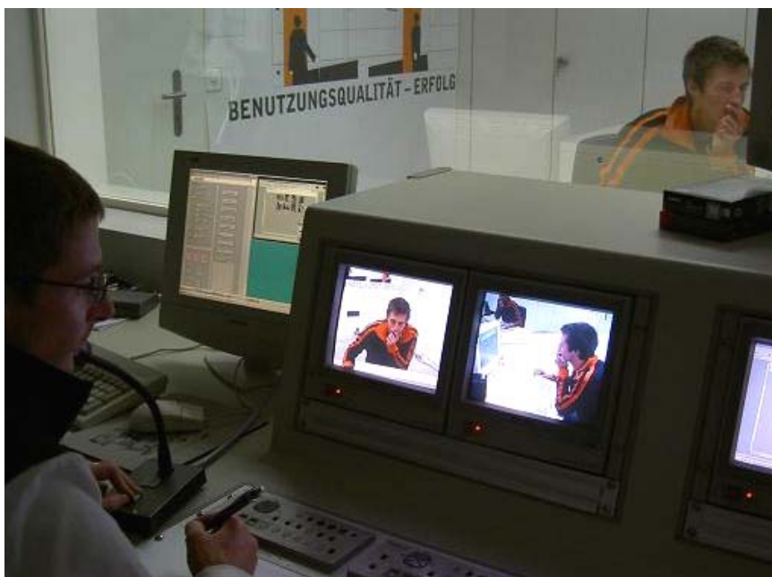
Fig.1: Set-up of the usability-lab (ergonomie & technologie GmbH): The test chamber is equipped with two video cameras. A one-way mirror window separates the control room from the test chamber. Thus the subjects can be observed without getting distracted by the observers.
